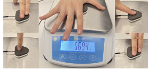
(b) Different modes of contact for data collection; Two fingers laid flat (top left), index fingertip (bottom left), palm (middle), one finger laid flat (top right) and two fingers pressing at an angle to emulate a combination of both normal and shear forces
